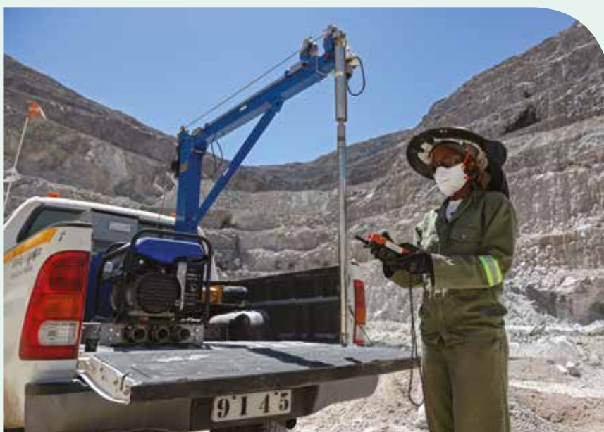
(Above) Faustina Shuuya (Senior Assistant Geological) using the 'down-the-hole' (DTH) logging technology at blast holes in the open pit to collect radiometric data down the holes with the use of wireline technology.
