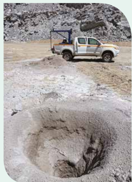
(Above) Faustina Shuuya (Senior Assistant Geological) using the 'down-the-hole' (DTH) logging technology at blast holes in the open pit to collect radiometric data down the holes with the use of wireline technology.
